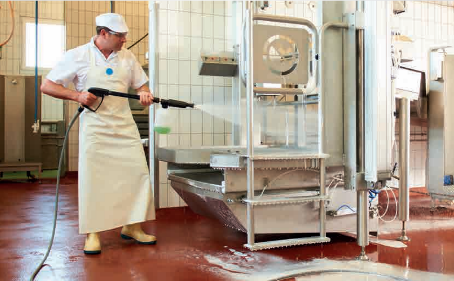
Fig. Trigger gun with safety catch with foam injector, page 75
